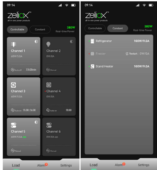
Figure 6: Controllable load interface and constant load interface
